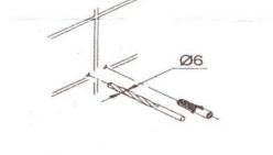
2. Drill holes for mounting brackets and insert anchors.
