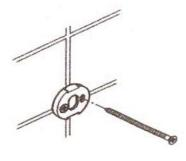
3. Screw mounting brackets securely to wall.
