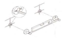
1. Hold accessory to desired location on wall. Mark wall for mounting brackets.
