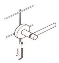
5. Secure accessory to bracket using set screws and allen wrench provided.
