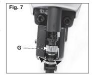
The adjustment knob has detents every full turn. Test drive another fastener and check depth. Repeat as necessary to achieve desired results. The amount of air pressure required will vary depending on the size of the fastener and the material being fastened. Experiment with the air pressure setting to determine the lowest setting that will consistently perform the job at hand.
