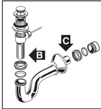
**8** Secure lavatory on hanger as shown in 5. Insert and tighten anchor screws if applicable. Connect hot and cold supply lines to the shut-off valves. Tighten trap joints for watertight assembly. Apply a bead of caulk around the edge which contacts the wall as shown.
