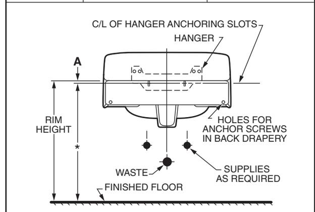
**3** Position hanger according to Step 2, making sure its center is aligned with the waste hole centerline. Mark the hanger screw locations through its mounting holes.
