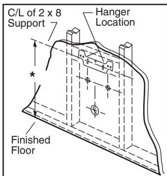
**2** Determine the desired rim height (for example 32") then select from the Table at right the height of the hanger mounting bolts centerline
