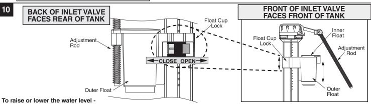
Turn water supply off, slightly loosen the both the supply coupling nut and valve lock nut. Be careful not to loosen to the point where water is leaking from the tank. Rotate the inlet valve clockwise to allow access to the float cup lock.
