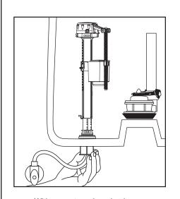
With correct washers in place (see Step 8a), tighten COUPLING NUT 1/4 turn beyond hand tight. DO NOT OVERTIGHTEN. 9
