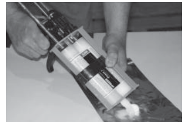
FIGURE 13: LEVELING THE PLUNGERS
