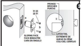
2) install latch so that the bevel (sloping face) on the latch bolt faces the strike lip
