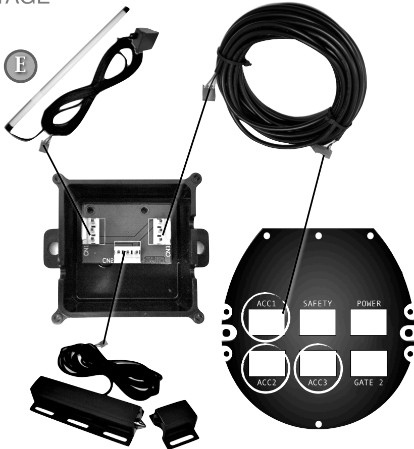
Figure E demonstrates how to “daisy-chain” Boerboel accessories together using the Low-Voltage Wire Kit. *Note: Boerboel Exit Wand Kit & Bolt Lock Kit shown as accessory examples.
