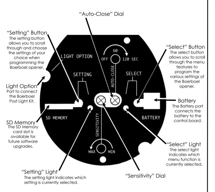
The "Auto-Close" Dial allows you to adjust the "Auto-Close" timing of the Boerboel opener. For dual gates, the "Auto-Close" Dial of the **Primary** opener will set the auto-close timing for both openers.
