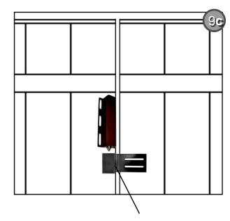
The Bolt Lock Receiver double acts as a positive stop for dual gates.
