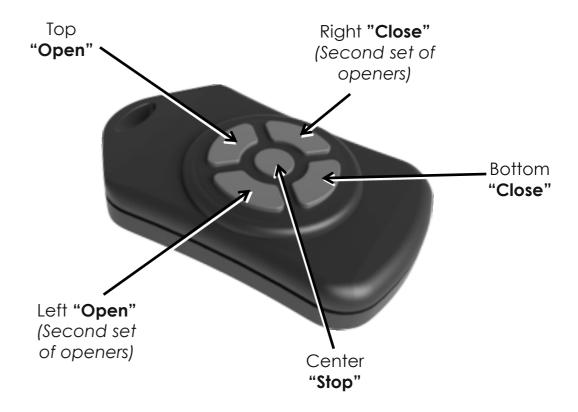
**Tip:** Any new wireless device that is learned during a later programming event will erase all previous devices and must be re-programmed. To save time, program or learn all wireless accessories at one time. The connection between the primary and secondary opener will not reset when devices are trained.
