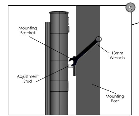
The MAX adjustment per Adjustment Stud is 1 3/4". **Do not over-extend.**
