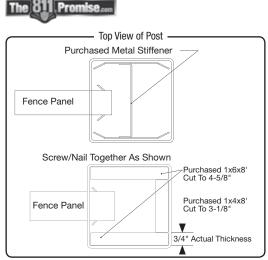
Post Spacing will be determined by gate width and hardware.
