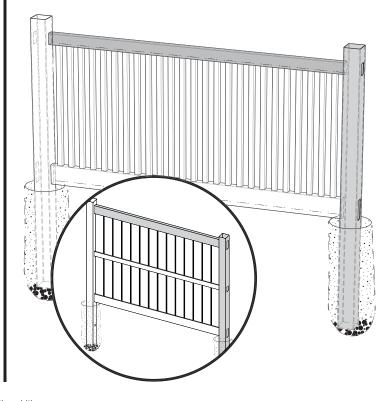
Check to ensure the second post is level , then add panel width plus one half the width of your post. This will locate the center of your next hole. Then dig the third post hole accordingly.
