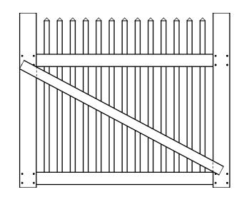
7.) Screw gate brace to pickets in 4 to 5 locations (depending on gate style) with square drive pan head screws.
