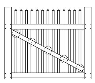
8.) Attach upright caps, install hinges and hang gate according to hinge instructions.
