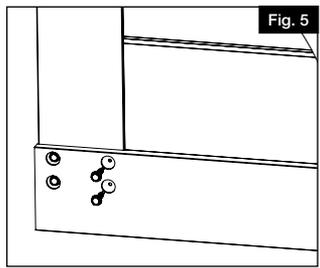
**7** Install screw hole plugs in all four corners. Install upright caps (Fig. 6).
