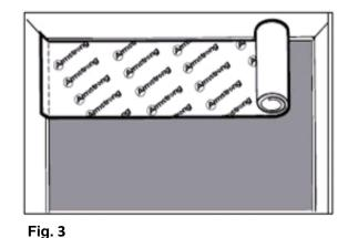
2. Place additional sections with butt seams as the installation progresses. If subfloor is concrete or for any existing floor over concrete, tape the seams with clear plastic tape (Fig. 4).
