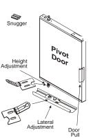
Both top and bottom pivot brackets can be adjusted laterally. For lateral adjustment release pivot bracket screw and slide pivot bracket along track, once located, re-tighten screw. Height adjustment is achieved by lifting door slightly and turning the bottom pivot with the aligner wrench as shown. Attach the door pull onto the pivot door at desired height (approx. 40" (1016mm) from
