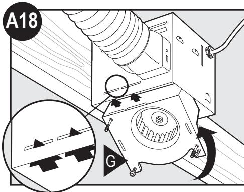
**ENG** Reinstall the motor by inserting the tabs and pushing up into position. Make sure the wires are not pinched between the motor and the housing.
