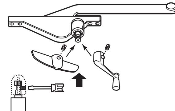
Loosen set screw on new handle and press onto stem, turning slightly until handle drops in, tighten screw.
