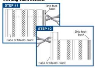
**STEP #1**: When cutting Shield sections, start from Drip Foot (back) and cut towards the hook area. Stop cutting before the hook.
