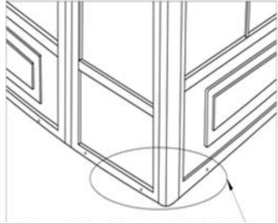
On the outside face, it is suggested to drill holes at the bottom end of the panels to permit drainage when installing on concrete floor
