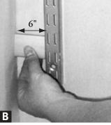
Position at 6" Position both outside uprights 6" from the right and left corners by using the 6" rail cover for spacing.
