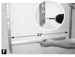
Use 22" rail cover for spacing Hang another 47.5" upright on the rail and use one of the 22" rail covers to space over 22". Drill 1/8" pilot hole and fasten screws in bottom hole. (Use wall anchor and 3/8" bit if there is no stud.) Place 22" rail cover over rail between uprights. Repeat step F for additional upright (if space allows).
