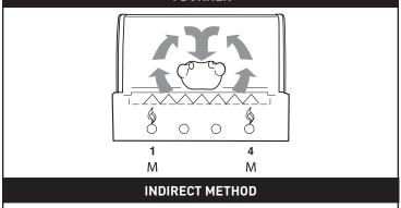
Food is placed on the area of the cooking grates between the lit burners
