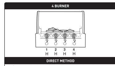
Food is placed on the area of the cooking grates directly over the lit burners
