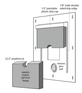
**STEP 1** - Detach bottom half of block from plastic flange by placing finger through 1" hole and then pulling down and out until block is detached. Remove remaining glue pad from the face of the plastic flange.
