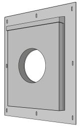
**STEP 2** - Flash all sides of block covering the nail flange. Install siding and caulk sides and bottom of block.
