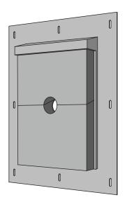
**STEP 2** - Feed water spigot or other application through the rectangular flange hole. Slide bottom half of block back up until tight. Face nail with 2" brad nails. Do not caulk 22.5° weathercut edge.
