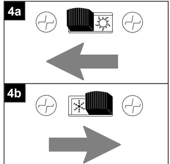
4b. In **cooler** weather, setting the reverse switch in the RIGHT position will result in upward airflow that can help move stagnant, hot air off the ceiling area.
