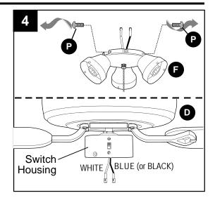
Connect WHITE wire from switch housing to WHITE wire from light kit fitter (F). Connect BLUE (or BLACK) wire from switch housing to BLACK wire from light kit fitter (F). Make sure molex connections are secure.
