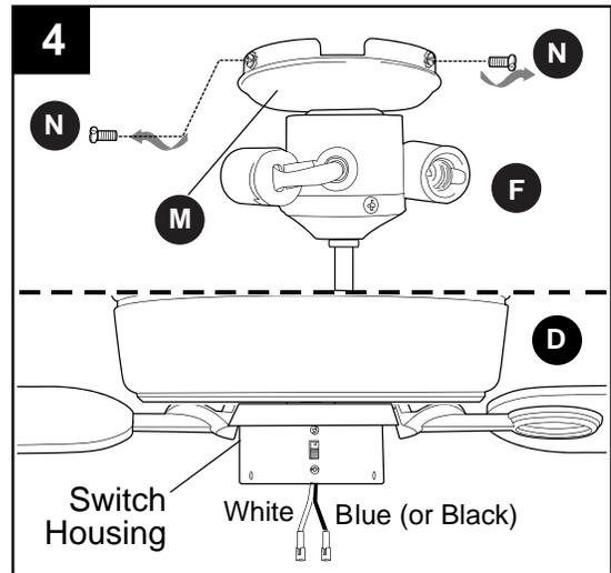
5. Connect WHITE molex wire from switch housing to WHITE molex wire from light kit fitter (F). Connect BLUE (or BLACK) molex wire from switch housing to BLACK molex wire from light kit fitter (F). Make sure molex connections are secure.
