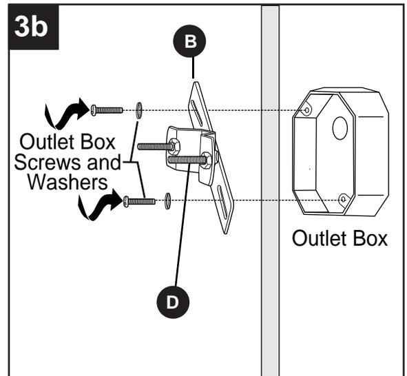
4. Adjust screws (D) to proper length by screwing them completely into mounting strap (B).
