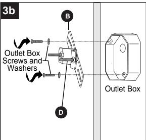
4. Adjust screws (D) to proper length by screwing them completely into mounting strap (B).
