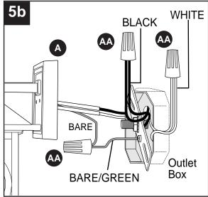
6. Wrap electrical tape (not included) around each individual wire connector (AA) down to the wire.
