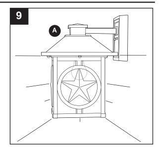
10. After completing installation, caulk fixture(A) mounting surface with silicone weather sealant (not included).
