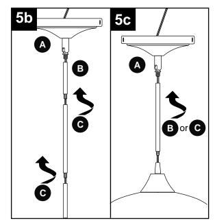
Depending on the number of rods used, you may need to cut the excess wire. You will need at least 10 inches of wire to work with.
