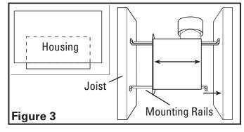
Mounting Tab Installation: Using the gauge on the fan's housing, line up housing so that it will be flush with the finished ceiling. Position the fan so that the tabs rest flat against the joist and secure with four nails (not provided) to ensure proper installation (Figure 4).
