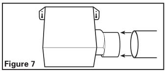
**NOTE:** If damper detaches from unit, reattach by snapping the collar back onto the unit. It is designed to only fit one way.
