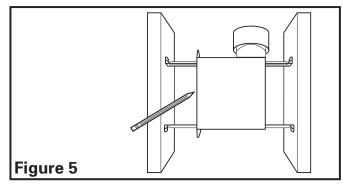
Mounting Tab Installation: Position housing against the joist and trace an outline of the housing onto the ceiling material (Figure 6). Set housing aside and cut opening, being careful not to cut or damage any electrical or other hidden utilities. Place housing next to the joist and insure that it is flush with the finished ceiling. Secure with four nails (not provided) to ensure proper installation (Figure 4).
