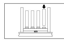
Step 4: Place the bottom rail between the rail posts, supported by a 3" block (2x4 scrap material works best). Secure rail to posts using Deckorators rail connectors (sold separately). Insert one Scenic Baluster into each baluster connector.
