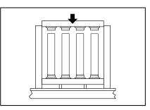
Step 5: Carefully place top rail over the balusters, making sure each baluster is seated properly in each baluster connector. Inspect finished railing for proper baluster spacing and secure top rail to posts. Attach support blocks to the bottom of the lower rail an equal distance from each post.
