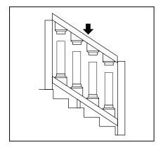
Step 8: Attach bottom rail to post. Insert one Scenic Baluster into each baluster stair connector. Carefully place top rail over the balusters, and secure top rail to post.
