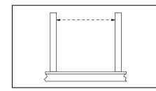
Step 1: Measure railing opening from post to post to determine the length of each rail section.
