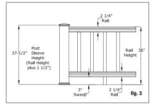
**Step 10** Determine the length of the balusters. Figure 3 illustrates how a 36"-high railing might be sized. Starting with a 3" sweep + 2" for the bottom railing, 29" baluster height + 2" for the top rail = a 36" rail height. Use 29" balusters for a 36" rail height. Use 35" balusters for 42" railings. If you want to have your railing at a different height, use figure 3 as a planning tool to determine the height to cut the post sleeves and the balusters.
