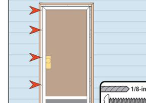
**6f** Cut extender weather stripping to length, peel adhesive backing and install.
