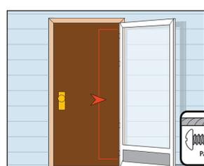
**4f** Push door tight against door frame, then pre-drill holes and install screws on the outer side of hinge rail starting with the top screw. Do not over tighten screws.
