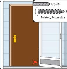
**4d** Slide rail extender to sill. Loosen hinge rail screw as needed, and retighten screw after lowering extender.
