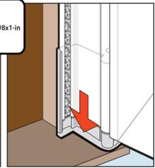
**4e** Pre-drill holes and place screws on the inner side of hinge rail in all 8 locations. Do not over tighten screws.
