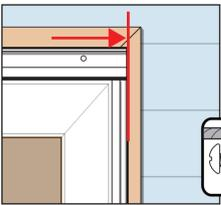
**5c** Pre-drill holes and install screws.
