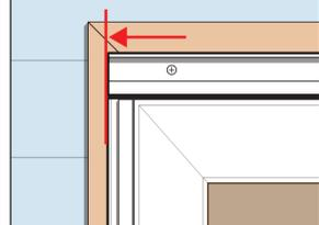
**6e** Pre-drill holes and fasten the latch rail with screws.
