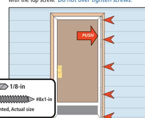
**4g** Cut extender weather stripping to length, peel adhesive backing and install.
