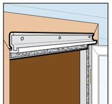
**5b** Close door to verify consistent clearance. Align drip cap to end of hinge rail.
