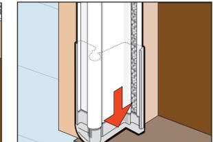
**6d** Align outside edge of latch rail with outside edge of drip cap. Verify that the door closes freely without hitting the latch rail.
