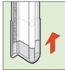
**4b** Hang storm door onto door frame using the placeholder screw. The door will settle approx. 1/16-in down. Tighten screw while pushing top of hinge rail tight against the door frame.
