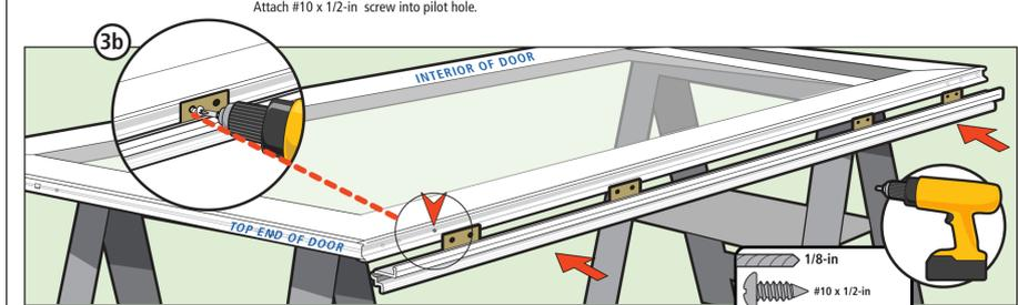
**3b** Locate factory installed hinge locator hole near top end of door, and place hinge rail as shown. Attach #10 x 1/2-in screw into pilot hole.
