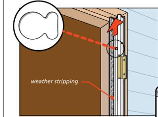
**2b** Use FIRST hole from top only. Mark hole with pencil, remove hinge rail, pre-drill and attach placeholder screw as shown. Do not tighten all of the way.
