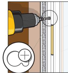
**4c** Pre-drill hole and install screw on the bottom outer side of hinge rail to secure door in opening. Do not overtighten.
