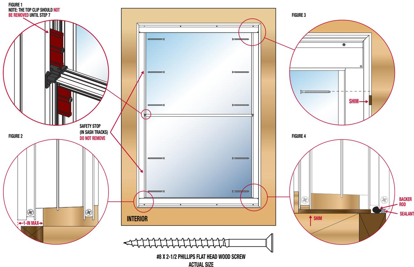
1. With the panel standing upright, remove and discard the two lower plastic shipping clips that are located under the top sash on the outside of the panel. **DO NOT** remove the clip on the inside located on the top of the bottom sash near the sash lock or the safety stops in the tracks.
