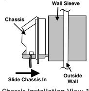
3. Slide the chassis into the wall sleeve until the chassis flanges contact the front edge of the wall sleeve.
