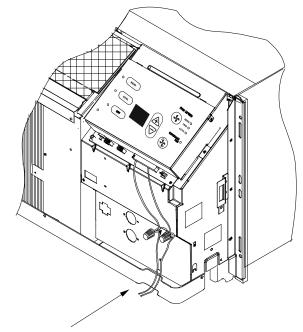
No holes are permitted in chassis basepan or wallsleeve when routing low voltage wire. Route the low voltage wires through the indention on the front of the basepan.
