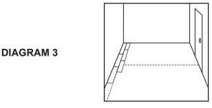
D. Continue to set each row wall to opposite wall, until room is complete. Use a matching molding at doorways where flooring does not continue to an adjoining room.
