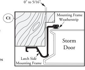
Hint: Drilling and installing the top screw first makes it easier to align the mounting frame correctly.
