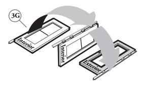
H. **Matching the angle of your entryway sill,** cut the bottom of the hinge mounting frame to length.
