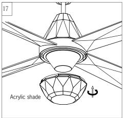
Attach Acrylic shade by locating dimples in light pan with grooves on the Acrylic shade and twist clockwise until tight.
