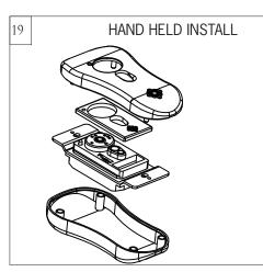
Place battery cover over battery compartment and buttons. Place remote over 2 pins on front cover. Attach cover of remote by placing over 4 pins and snapping into place.
