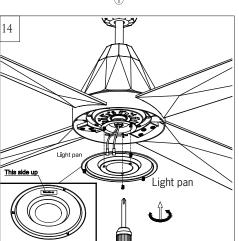
Attach light pan onto the plate on motor, aligning the keyhole slots on the light plate with the preassembled screws on the plate. Twist clockwise till lock. Reinstall the screw removed in step 13. Tighten all screws securely. **Note**: Make sure the side with a label "This side up" is installed upward.
