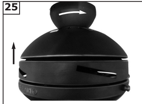
Lift fan to mounting bracket, aligning the "L" shape holes with the screws on the mounting bracket. Turn the fan clockwise to lock in position. Install the other 2 screws included in hardware bag and tighten all 4 securely.
