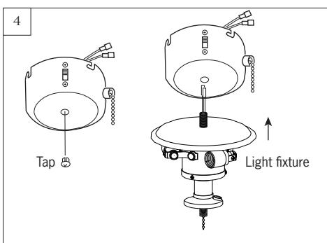
Remove tap from bottom of switch housing. Thread lead wires from light fixture through central hole in switch housing and then install switch housing onto light fixture by turning clockwise till tight.
