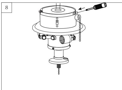
Install light kit assembly (switch housing) onto the fan with set screws removed in step 2.
