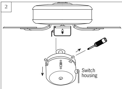
Remove set screws from switch housing. Keep screws. Switch housing may be different than shown.
