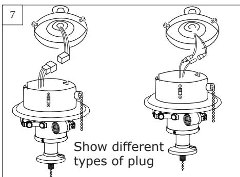
Lift light fixture assembly up, connect the plug from fan to the plug from light kit assembly. Make sure the plugs are clasped firmly.
