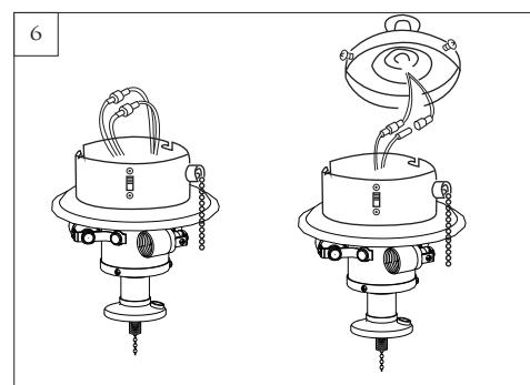
Connect white wire from light fixture with white wire from switch housing (or fan) and then connect black wire from light fixture with black (or blue) wire from switch housing (or fan).
