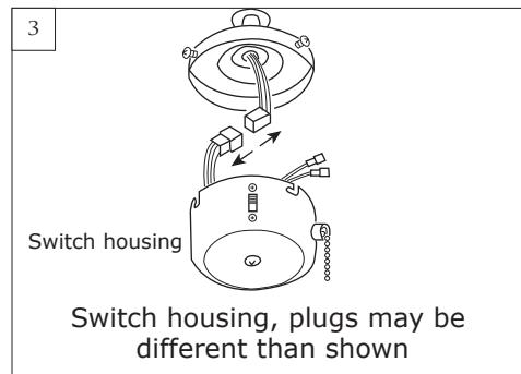
Unplug (If wiring with plugs) and remove the switch housing from fan.
