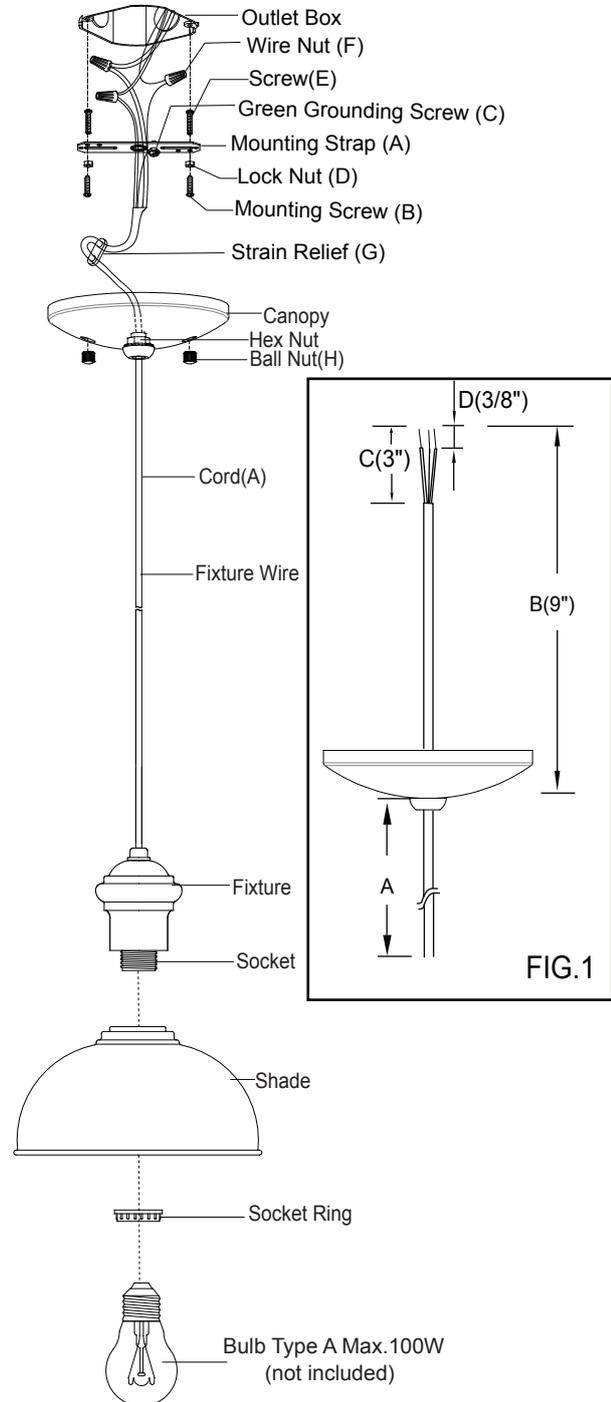
9. Attach shade to fixture, then secure it with socket ring.
