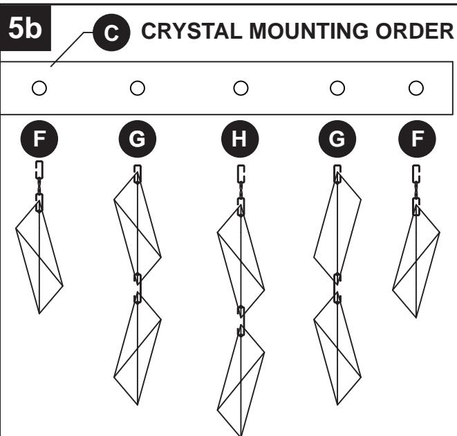
5. Hook crystals strings (F-G-H) onto mounting surface (C).
