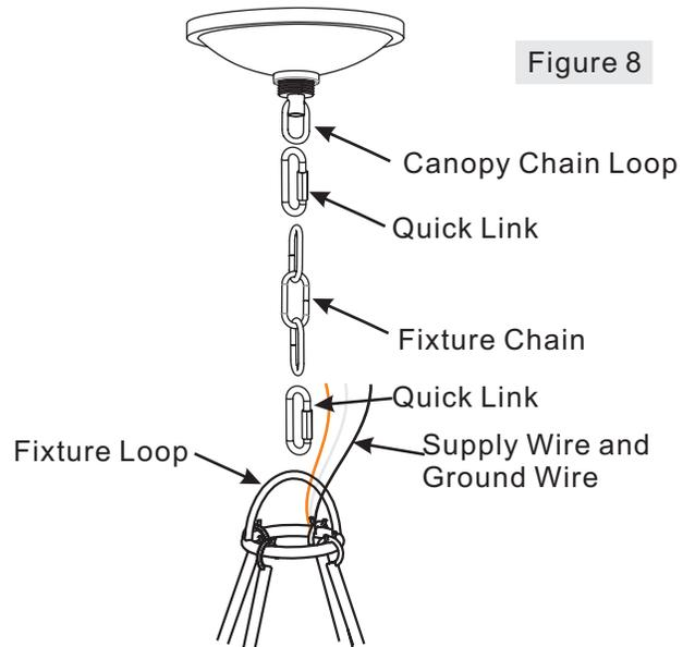
**STEP 9 – Pass Supply Wires through Fixture Chain**
