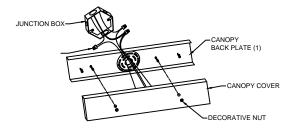
Reinstall the canopy cover, making sure to tuck the excess lines into the canopy. Install the recommended bulb in the socket, and then install the lid (shade/cover) of the decorative fixture to each light(arm), using the supplied screws or decorative nuts.
