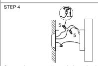
Connect the power and neutral wires using the provided wire caps. Connect the white wire from the fixture to the neutral wire in your ceiling junction box. Connect the black wire to the power wire in your ceiling junction box. Connect the bare copper ground wire to the green screw on the hanger.
