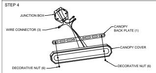
Install the recommended bulbs in the sockets and then install the canopy (shade/cover) of the decorative fixture to the mounting hanger, using the supplied screws or decorative nuts (6).
