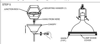
Install the recommended bulb in the socket, and then install the canopy (shade/cover) to the mounting hanger by hanging it on the hook. Slide the canopy up until it touches the ceiling and tighten the screw with a phillips head screwdriver as shown above. Install the lamp shade cover by threading the knobs around the sides by hand pressure.
