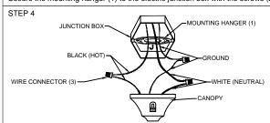
Connect the hot wire from main wire to the hot wire from power supply. Connect the neutral wire from the main wire to the neutral wire from power supply. Fix the ground wire from fitting to ground wire (grounding) from power supply.
