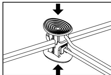
4.2 Align and fit the main low voltage cable vertically to the slot of wire connector as shown.
