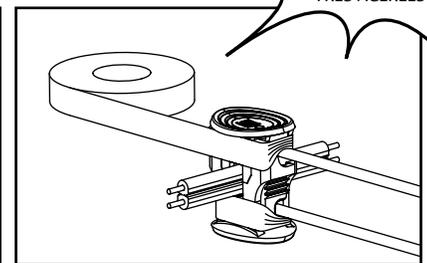
4.3 Press the wire connector together until fully seated and locked around the cable. Pre-set prongs will pierce the cable insulation and establish contact. Turn on the power unit. If the light fixture does not turn on, repeat operations 4.2 and 4.3.
