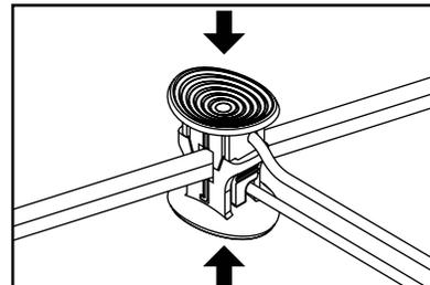
**4.3** Press the wire connector together until fully seated and locked around the cable. Pre-set prongs will pierce the cable insulation and establish contact. Turn on the power unit. If the light fixture does not turn on, repeat operations 4.2 and 4.3.
