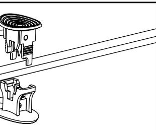
**4.2** Align and fit the main low voltage cable vertically to the slot of wire connector as shown.
