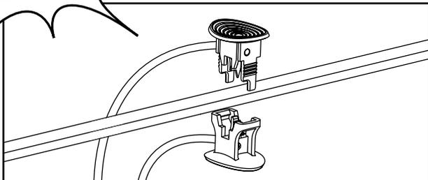
**4.1** Place the wire connector on opposite sides of the low voltage cable where the fixture will be located.
