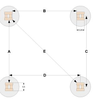
(Suggested for installation on lawns with poured concrete footings. For other surfaces, appropriate mounting methods should be used)
