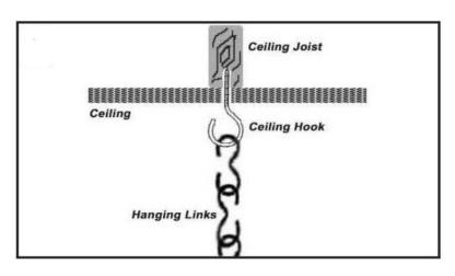
Photo D - Proper Installation
