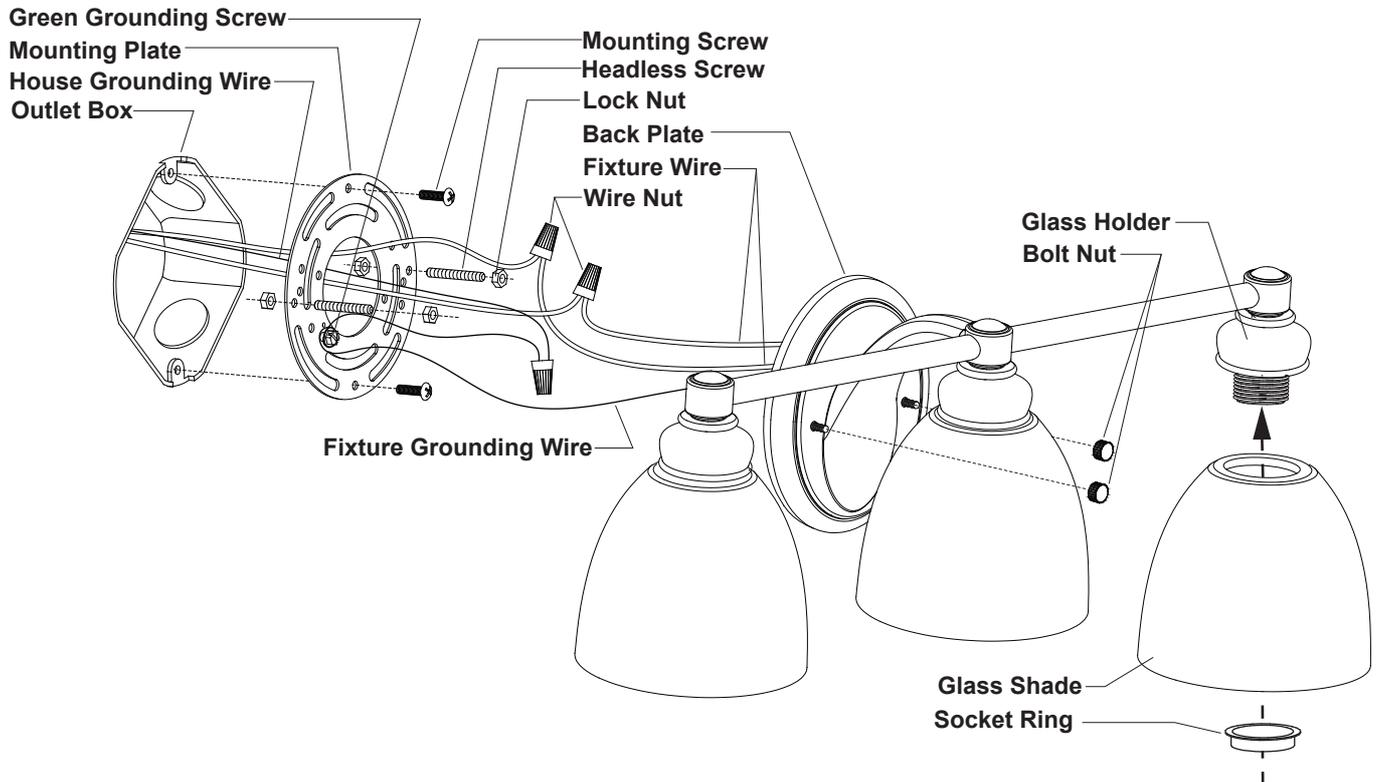
1. Thread two headless screws to the mounting plate, and secure them with four lock nuts (two on each side of the mounting plate). Adjust the length of the headless screws if necessary.
