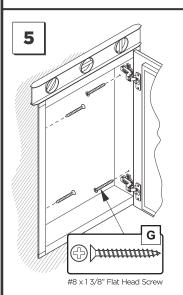
Level, then secure the cabinet with screws (G) through the mounting holes into the framing studs.
