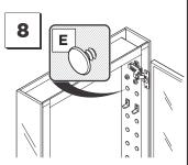
Fill remaining holes with the plugs (**E**).
